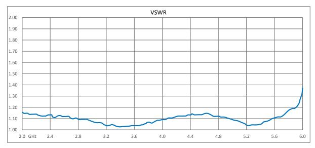
Click the following link (or enter part number in "SEARCH" on website) to obtain additional part information including price, inventory and certifications: Type N F/F Bulkhead Coaxial RF Surge Protector, 2GHz - 6GHz, DC Block, 10W, IP67, .5uJ, 10kA, Filter AL-LSXM
